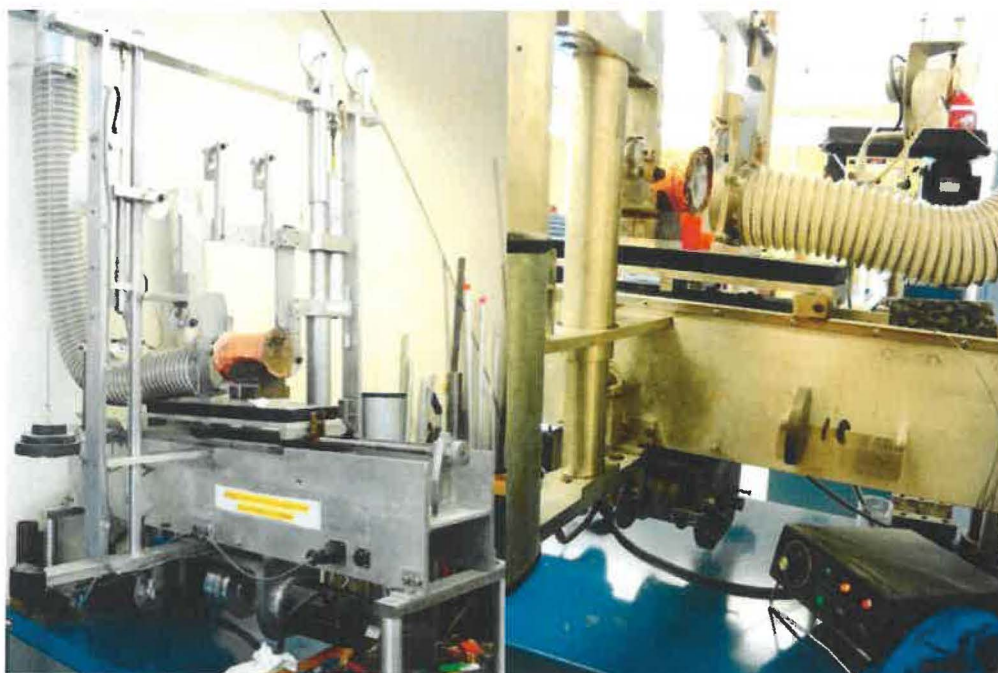
Figure 6. Diamond wire saw with ventilation, pulley system, adjustable table, wheel, pump and pump controller
